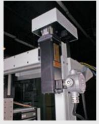
Heavy-duty servo motors for precise, repeatable motion. (Explosion proof & dust tight wiring available.)
