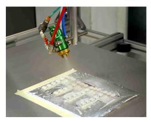
as it does horizontally. The forces acting on tiny paint droplets along with air currents in the paint booth often end up having unintended effects. What looks good in the lab may not look the same on the production line. One of the largest manufacturers of industrial and automotive coatings had exactly that concern; to make the lab process as close to reality as possible.
