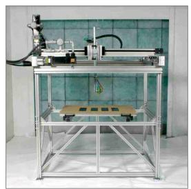
which can be tuned to accurately simulate real-world line conditions in the lab. "The PanelPro-H machine has the same Windows based control architecture as our other machines" says Artomation engineer Chuck Greene. "This software allows the customer to create a trajectory and spray profile that mimics what will happen in production. We've been doing this for years now in the vertical world. But for our customers who paint horizontally this provides a solution for them as well."
