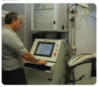
The system includes three servo-driven axes of motion, each of which is controlled through the machine's Windows-driven computer interface.
