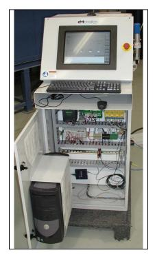
The ARTomation controller is the central brain of a complete precision coating system. It is designed with components having the highest level of operational reliability. The electronics and drives are mounted in a shielded steel cabinet, protecting the components from dirt and dust in the plant atmosphere.
