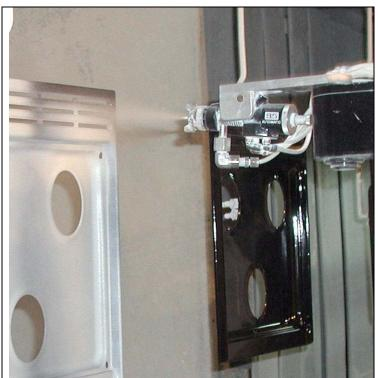
An Artomation 3 axis upright gun mover applies a porcelain color coat to stove tops providing savings in both labor and material
